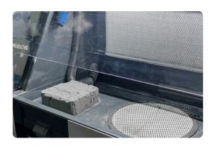
4. Extracting parts: This step is sure to bring back childhood memories of the sandbox! An included set of brushes and picks of varying sizes helps scrub and scrape powder out of even the tiniest of features. Chunks of powder can be easily broken up by hand or scrubbed off with the included large brush. A wire basket is provided to neatly collect your parts while you continue processing a print.
